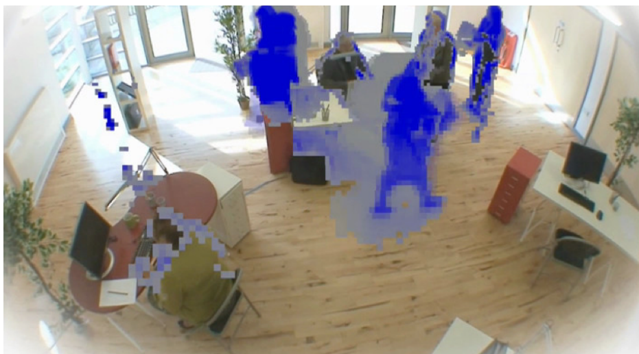
Sample screen shot shows use of Hitachi Video Analytics' Privacy Protector feature: HVA automatically detects and masks people's images with full body pixelation and/or color masking.
